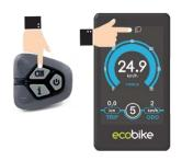
With the turned on display, click on / off at once the lights button to turn on the display backlight and the front and rear lights. Click the button again to turn off the backlight and lights. When the light is on, you can see the icon on the screen as in the picture beside.
