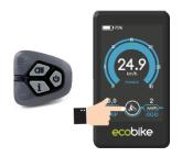
Press and hold the "MINUS" button to start the motor that will go at 6km / h without pedaling. The display will show the icon as in the picture beside. When the user releases the button, the engine will automatically shut down.
