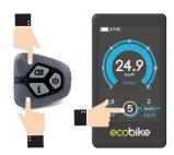
The level of electric assistance can be adjusted using the display. Adjustments can always be made while driving. The electric system has 6 levels, depending on them the speed to which the bike will accelerate. The default assistance level after turning the display on is "1". To change the assistance level, use the "PLUS" buttons to increase the assistance level or "MINUS" to decrease the assistance level, respectively.
