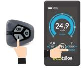
When the electrical system is turned on, the display will show the speed and distance as defaults.
